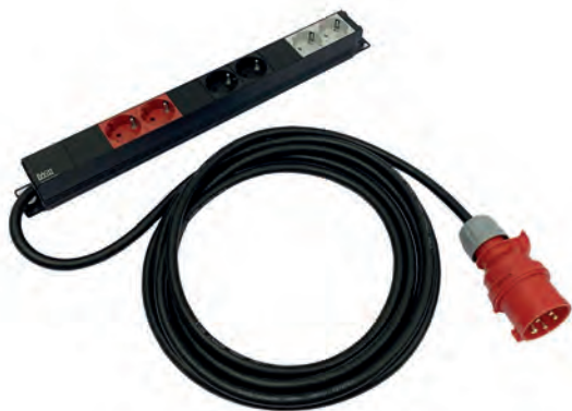
plugbar_ CEE_400V_3x16A_3600W Item No.: 11162
